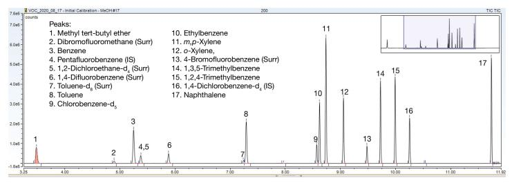
Figure 2. Total ion chromatogram of a methanol extracted 5 g spiked baked sand sample containing a final concentration of 200 ppb (µg/L) PVOC/GRO Mix (Wisconsin)
