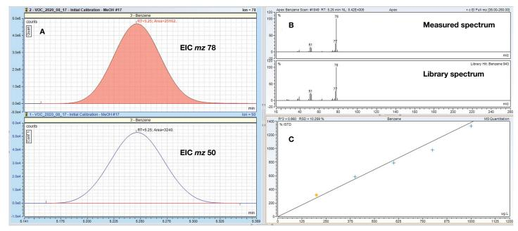
Figure 5. Chromeleon CDS results browser showing extracted ion chromatograms (quan ion *m/z* 78, confirmatory ion *m/z* 50) for benzene in the methanol extract of 5 g baked sand sample containing a final concentration of 200 ppb PVOC/GRO Mix (Wisconsin) standard, quantitation ion and one confirming ion (A), a matching measured spectrum to the NIST library (B), and a linear calibration over a concentration range of 200 ppb to 1000 ppb (C)
