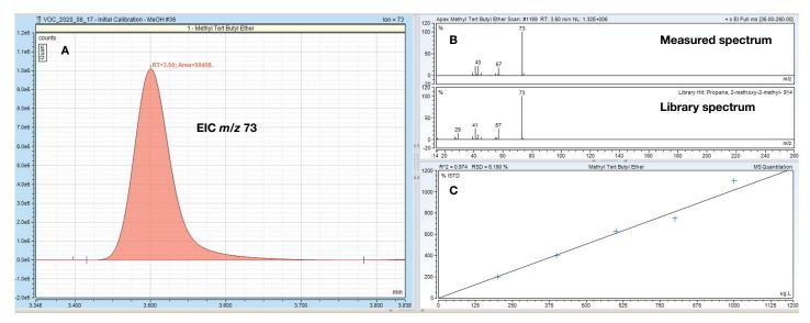
Figure 4. Chromeleon CDS results browser showing extracted ion chromatogram for methyl tert-butyl ether (MTBE) (*m/z* 73) in the methanol extract of 5 g baked sand sample containing a final concentration of 200 ppb PVOC/GRO Mix (Wisconsin) standard, quantitation ion (A), a matching measured spectrum to the NIST library (B), and a linear calibration over a concentration range of 200 ppb to 1000 ppb(C)
