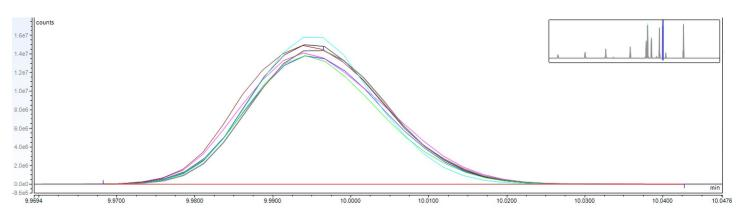
Figure 3. Total ion chromatogram of (n=7 replicates) of 1,2,4-trimethylbenzene in methanol extract of 5 g spiked baked sand sample, containing a final concentration of 600 ppb PVOC/GRO Mix (Wisconsin), displaying good reproducibility with a 5.3% RSD and a 114% recovery
