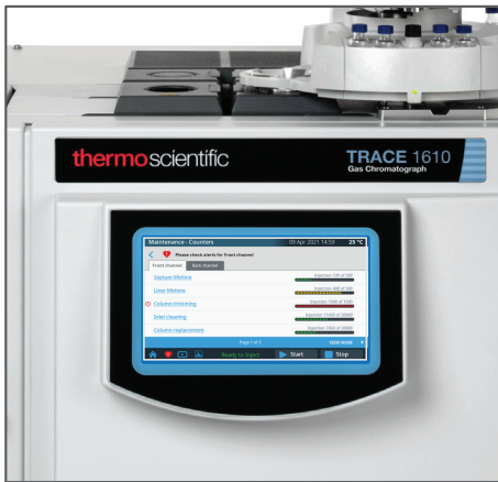
Figure 3. Consumables usage tracking on the TRACE 1610 GC touch screen
