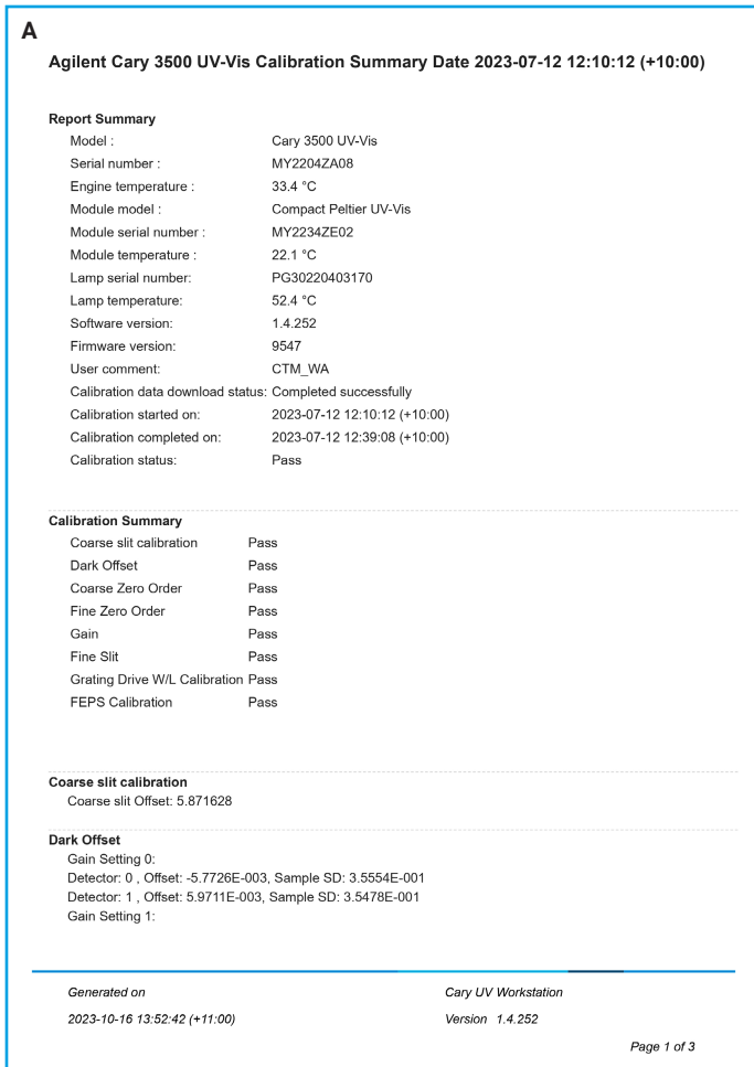
Figure 3. Calibration routine detailed report (A) and self-test detailed report (B).
