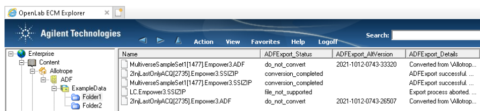
Figure 7. OpenLab ECM folder with changed display settings to visualize the user defined keys. Two of the three example SSIZip archives are converted to ADF and the ADFExport_Status is set to “conversion_completed”. For LC.Empower3.SSIZIP the export to ADF is not supported and the ADFExport_Status is set to “file_not_supported”.
