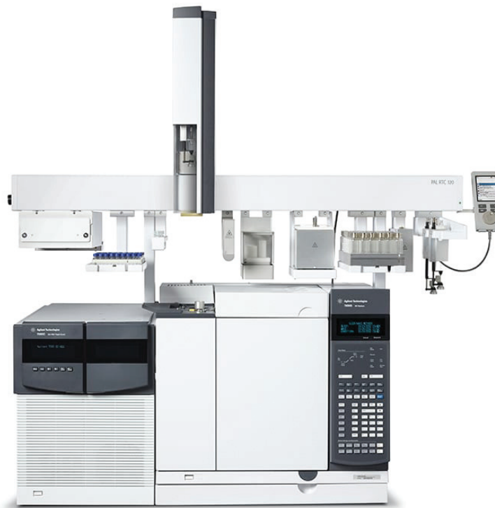
Figure 3. The PAL RTC rail system combined with an Agilent 7890B GC and an Agilent 5977B GC/MSD.
