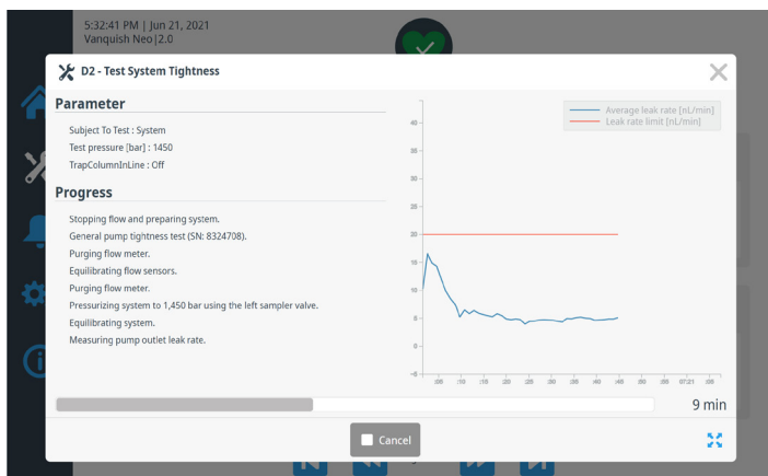
Figure 7. The “Test System Tightness” script performs a system-wide or module-specific test to check for leakages at a user defined pressure. When applicable, the trap column can also be included in the test.
