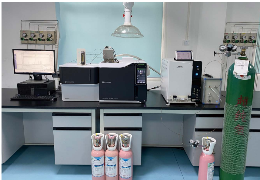
Nexis GC-2030 and SCD-2030 installed in the Hydrogen Energy and Fuel Cell Analytical Method Work Group lab
