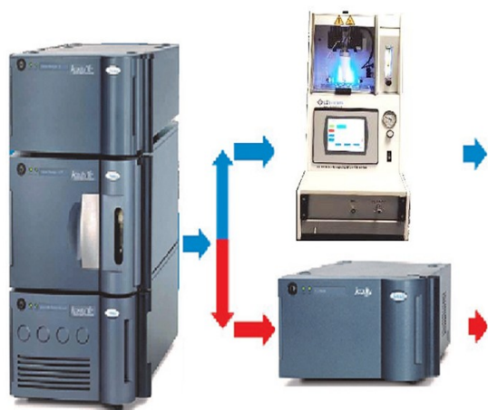
Figure 1. Waters ACQUITY APC SEC Core 1 System with post column split flow to the ACQUITY RI Detector and the HTX Technologies LC-Transform 700 sample collection system.
