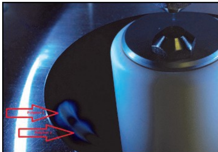
Figure 3 The above image is the germanium collection disk in the HTX LC-T 700. The two spots identified by the red arrows indicate the deposit of the two narrow polystyrene samples collected (top 55000 Da bottom 31000 Da).
