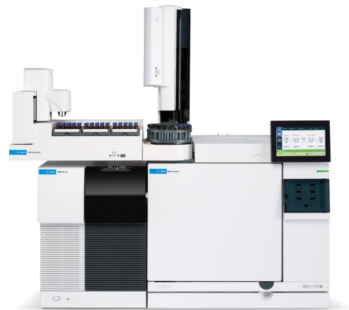
Figure 2. Agilent 8890 GC with Agilent 7000D QQQ used for this analysis.
