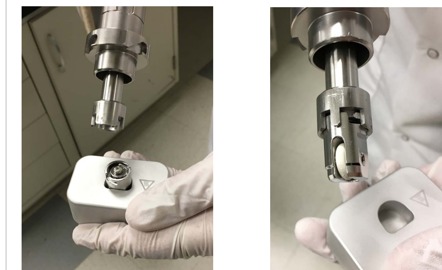
Figure 7. NeverVent technology hardware and mechanism of vent-free column replacement.
