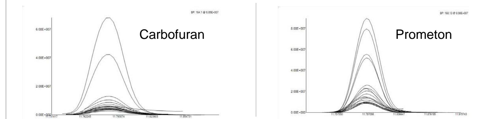
Figure 6. Deconvolution plugin result showing all the binned XICs associated with individual compounds.
