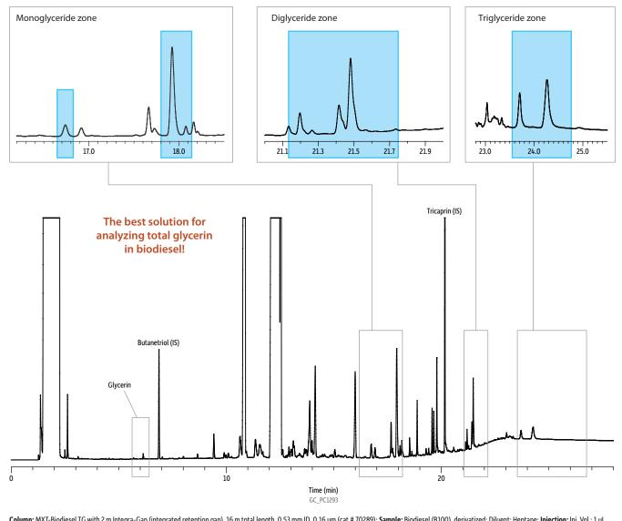
Column: MXT-Biodiesel TG with 2 m Integra-Gap (integrated retention gap), 16 m total length, 0.53 mm ID, 0.16 µm (cat.# 70289); Sample: Biodiesel (B100), derivatized; Diluent: Heptane; Injection: Inj. Vol.: 1 µL cold on-column; Temp. Program: Oven track; Oven: Oven Temp.: 50 °C (hold 1 min) to 180 °C at 15 °C/min to 230 °C at 7 °C/min to 380 °C at 30 °C/min (hold 5 min); Carrier Gas: He, constant flow; Flow Rate: 3 mL/ min; Detector: FID @ 380 °C; Instrument: Agilent 7890A GC
