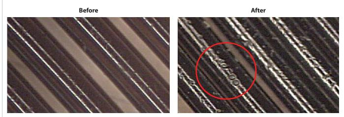
100 temperature cycles to 430 °C totaling 500 minutes at maximum temperature.
