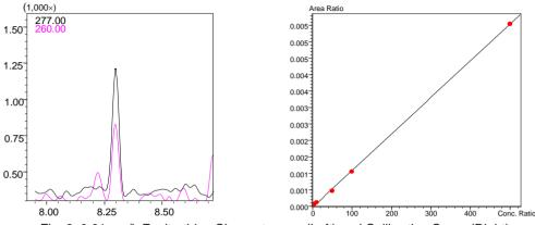
Fig. 2: 0.01 mg/L Fenitrothion Chromatogram (Left) and Calibration Curve (Right)
