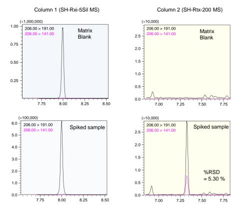
Fig. 2: MRM Chromatograms of Chloroneb in a Soy Bean Sample Using Column 1 (left) and Column 2 (right)
