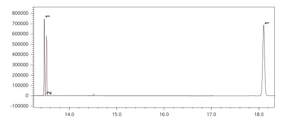
Figure 1 MRM chromatogram of organic tin pesticide derivatives (1.0 mg/L each)
