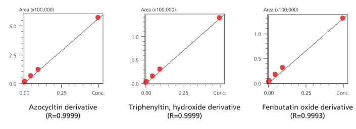
Fig.2. The calibration curve of organic tin pesticide derivatives
