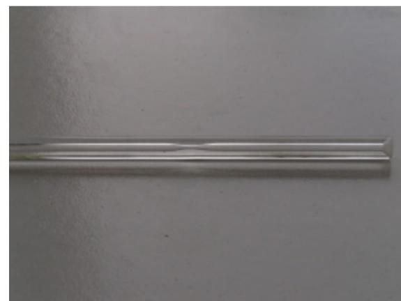
Fig 2: Liner for simple on column method
