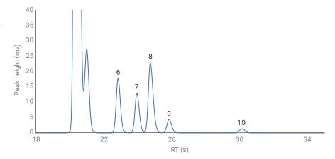
Figure 2. standard gas (simulated RGA) on PPU channel.
