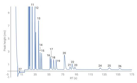
Figure 3. standard gas (simulated RGA) on Al<sub>2</sub>O<sub>3</sub> BF2D channel.
