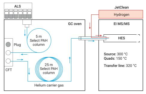
**Figure 2.** GC/MS/MS in electron ionization (EI) mode configured with BF and JetClean. Arrows indicate direction of helium carrier gas flow. CFT purged 3-way splitter is used to configure the two columns for BF. The JetClean self-cleaning ion source is configured to the MSD in Acquire and Clean mode to allow 0.33 mL/min of hydrogen flow to the source. ALS = automatic liquid sampler. HES = high efficiency source. CFT = Capillary Flow Technology.
