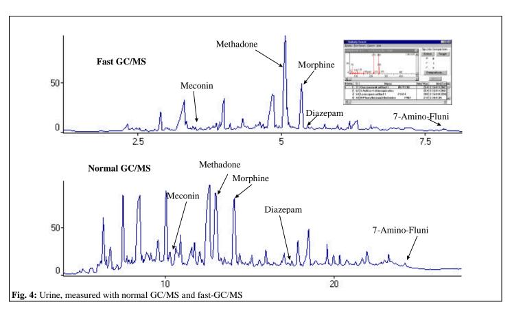
**Fig. 4** shows the difference between the fast GC/MS and the normal GC/MS. For this example the same urine was measured with both methods. In general, the analysis cycle can be decreased from 40 minutes to 14 minutes with fast GC/MS. The
