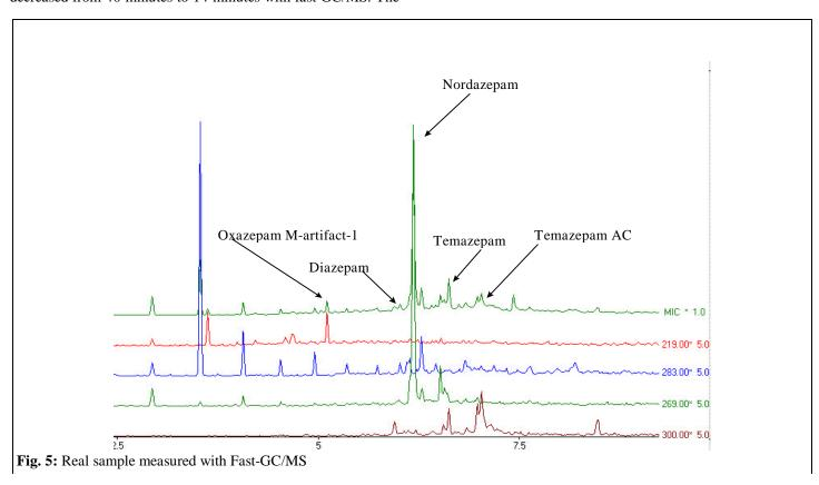
**Fig. 5** shows a drug urine with the identification of some of the relevant substances. It makes sense to work with Multi-Ion-Chromatograms, to ease the identification of the Benzodiazepines. All relevant substances could be identified with fast-GC/MS, which were previously detected with normal GC/MS.
