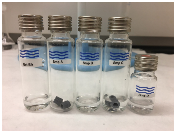
Figure 2. Samples prepared for extractable study from rubber plunger stoppers
