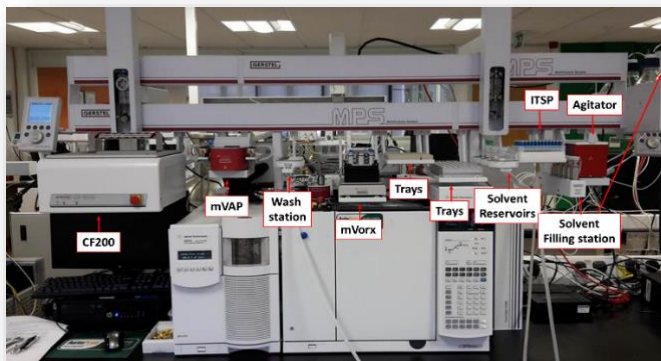
Figure 1: Anatune solution for fully automated opiates analysis in blood
