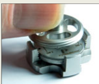
Figure 2. Installing the wafer in the holder
