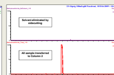
Figure 10. Chromatograms shown in Figures 8 and 9 plotted together at a larger scale to show the efficacy of sidecutting for solvent removal.
