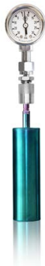
Figure 2 Testing sampler pressure in the field prior to sampling to ensure helium is still above 3 psig. Even Though helium may have dropped down from the initial 7 psig, the presence of any positive helium pressure is an indication that no air or contaminants have entered the sampler.
