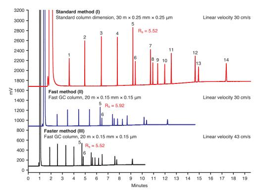
Figure 1: Chromatograms for FAME standard mix C8–C24 analyzed on a standard GC column and Fast GC column. Resolution values were compared on peaks 5 and 6.
