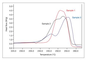
*Figure 3A.* The beta phase fusion effects of the systems 1, 2, and 3 (in 1993), i.e. heating rate 20 °C/min.
