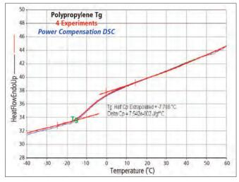
Figure 4. Reproducibility of Tg of reheat polypropylene sample showing overlay of four (4) DSC experiments.
