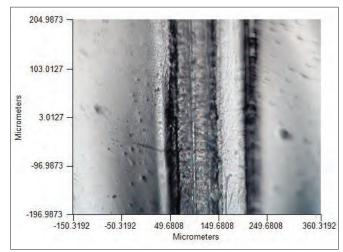
Figure 7: Visible image for multilayer food packaging material.
