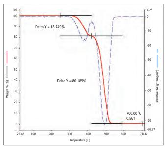
Figure 1. TGA curve generated from the analysis of EVA samples.
