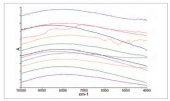
Figure 6. Near-IR reflectance spectra of black plastics.
