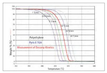
Figure 8. Effect of heating heat on the thermal decomposition of polyethylene.
