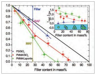
Figure 3. Calorimetric relaxation strength as a function of nanofiller content. The vertical double arrow indicates the amount of RAF for PMMA at 27 m% Laponite RD™ filler. Symbols:  $\triangle$  – PS with spherical SiO<sub>2</sub> nanoparticles;  $\bigcirc$  – PMMA with spherical SiO<sub>2</sub> nanoparticles;  $\bigcirc$  – PMMA with Laponite RD™ clay nanoparticles. The inset shows the percentage of the RAF versus filler content, see text.
