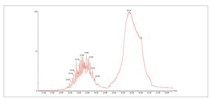
Figure 2. The MS analysis of the evolved gas generated during the TGA of EVA.
