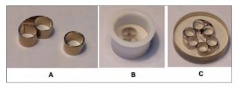
Figure 1. Fixing and embedding laminate samples.
