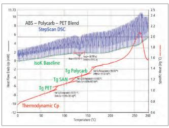
Figure 3. StepScan DSC results on polymer tri-blend.
