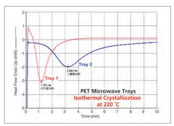
Figure 9. Overlay of DSC isothermal crystallization results at 220  $^{\circ}\text{C}$  for PET microwave trays 1 and 2.
