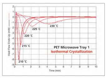
Figure 7. Isothermal crystallization results for PET Tray 1.
