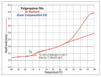
Figure 2. Enlarged view of Tg of as received polypropylene film sample.
