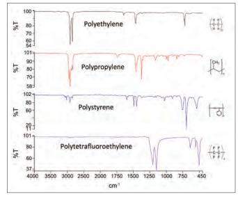
Figure 1. Mid-IR spectra of common polymers.
