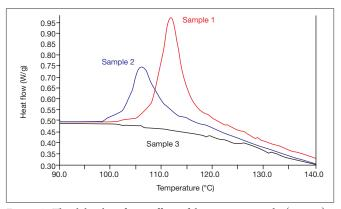
Figure 4A. The alpha phase fusion effects of the systems 1, 2 and 3 (in 1993), i.e. heating rate  $20\,^{\circ}\text{C/min}$ .
