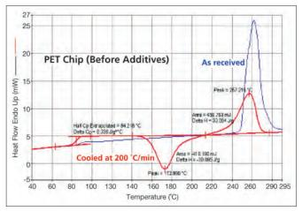
Figure 2. DSC results for PET chip (before additives) showing as received resin and resin after being melted and cooled at 200  $^{\circ}$ C/min.
