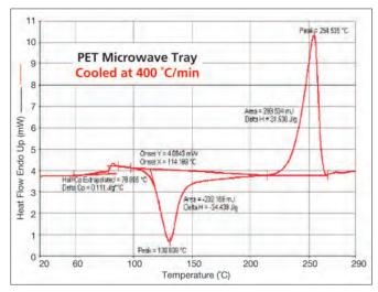
Figure 4. DSC results for PET tray resin after cooling at 400  $^{\circ}\text{C/min}.$
