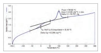
Figure 2. Specific heat capacity data for thermoplastic polyurethane composite using the 400  $^{\circ}\text{C/min}$  heat-cool  $C_{\text{P}}$  method, with  $T_{\text{g}}$  and peak calculations applied.
