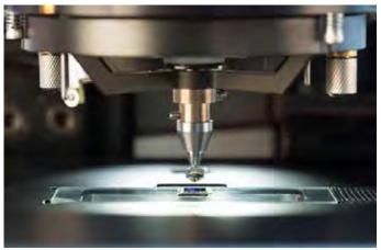
Figure 7: The automated dropdown ATR crystal.
