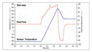
Figure 1. Raw data for thermoplastic polyurethane nanocomposite using the 400  $^{\circ}$  C/min heat-cool C<sub>p</sub> method – analysis time: 5 minutes.
