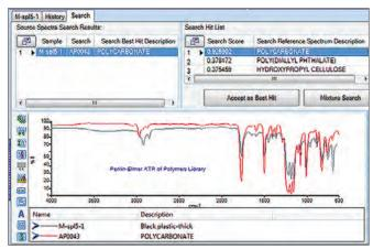
${\it Figure~10.}~{\it Sample~2~identified~as~Polycarbonate~base~material.}$
