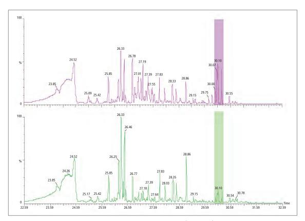
Figure 3. The GC/MS data collected during the TGA analysis of PVC with DINP (purple - top) and with a mixture of non-regulated phthalates (green - bottom). Differences are noted in peaks with tentative identification as phthalates around 30 minutes.
