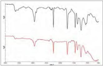
Figure 5: Reflectance spectra of the two contaminant fibers.
