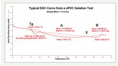
This curve shows a typical DSC curve for this type of analysis. The features seen are;
