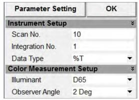
Figure 1. Parameter Setting of Color Analysis Mode.
