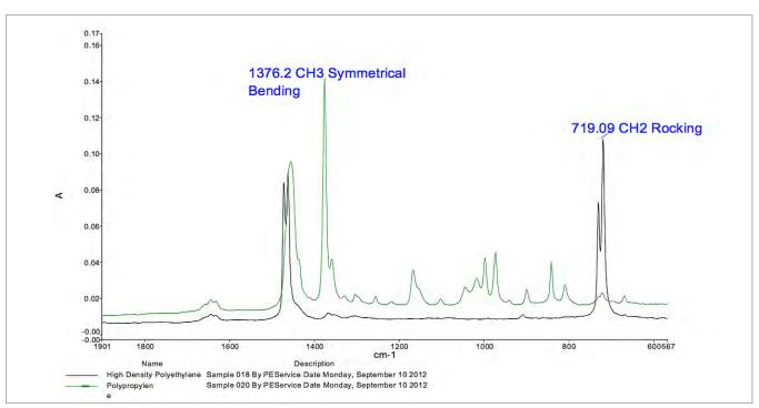
Figure 1. Spectral Comparison of High Density Polyethylene and Polypropylene
