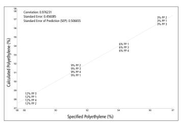
Figure 3. Calibration Model for PE
