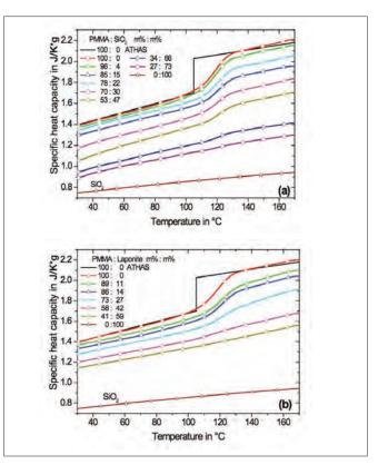
Figure 2. Specific heat capacity of nanocomposites in respect to sample mass. (a) – PMMA with spherical SiO₂ nanoparticles, (b) – PMMA with Laponite RD $^{TM}$ . Specific heat capacity for SiO₂ is shown too. The black lines represent reference data for PMMA from ATHAS⁴. Diamond DSC, StepScan mode.
