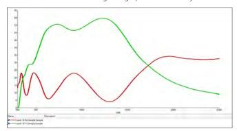
Figure 6. Transmission (green) and reflectance (red)spectra of thin film cyrstalline silicon acquired for absorptance determination.
