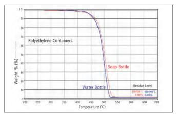
Figure 4. TGA degradation for two different HDPE bottles.
