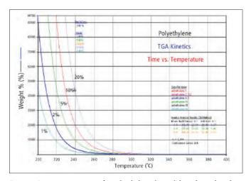
$\label{thm:polyethylene} \emph{Figure 9}. \ \ Isoconversion curves for polyethylene thermal degradation based on kinetics modeling.$
