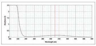
Figure 3. Spectrum of color formed for the determination of 'Formaldehyde' contents.
