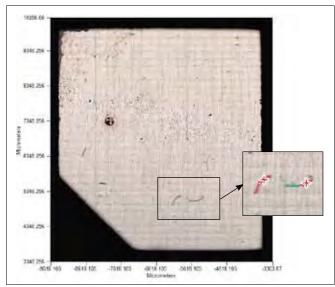
${\it Figure~4:} \ {\it The~Visible~Image~Survey~and~expanded~region~show~automatic~detection~of~contaminants.}$
