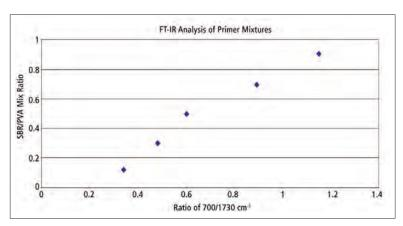
Figure 5. Calibration curve for the FT-IR analysis of standard mixtures of SBR and PVA. Peak height ratios are the SBR/styrene absorbance at 700 cm $^{-1}$  divided by the PVA/carbonyl absorbance at 1732 cm $^{-1}$ .
