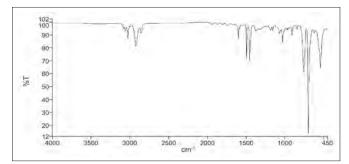
Figure 3. ATR spectrum of plastic sample.
