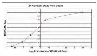
Figure 7. Calibration curve for the TGA analysis of standard mixtures of SBR and PVA. Calculated ratios are the SBR/1st derivative peak height at 425  $^{\circ}$ C divided by the PVA/1st derivative peak height at 350  $^{\circ}$ C.
