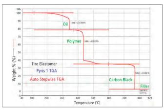
Figure 6. Auto Stepwise TGA compositional results for tire elastomer showing separation of oil, polymer, carbon black and filler.
