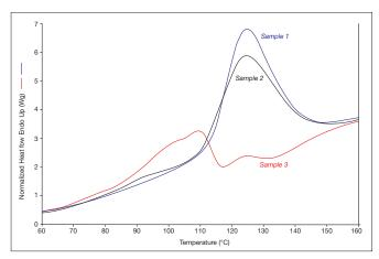
*Figure 4B.* The alpha phase fusion effects of the systems 1, 2 and 3 (in 2005), i.e. heating rate  $300\,^{\circ}$ C/min.
