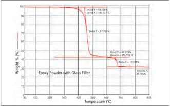
Figure 3. TGA results for epoxy-glass powder.
