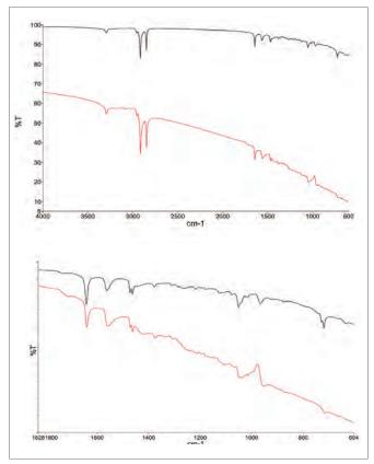
Figure 7. Spectra of carbon-filled o-ring on germanium crystal (upper) and diamond crystal (lower).
