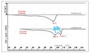
Figure 4. Polyethylene blend with different cooling rates.
