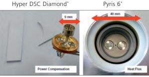
Figure 1. Furnace of HyperDSC versus heat flux DSC furnace.
