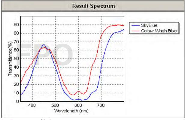
Figure 2. Transmittance spectrum of color filters.
