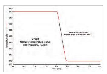
$\label{eq:Figure 3. Sample temperature vs. time profile of the isothermal crystallization experiment.$
