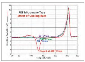
Figure 6. Overlay of DSC results on PET tray after cooling at rates of 400, 200, 100 and 50  $^{\circ}$ C/min.
