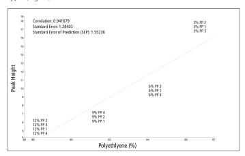
Figure 4. PE Calibration Plot of Peak Height vs Specified Concentration with Peak Ratio and Linear Regression Fit Type
