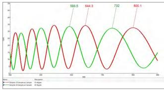
Figure 15. Silicon nitride thin film coating on a silicon substrate semiconductor wafer scanned in absolute reflectance at two different angles of incidence (red =  $15^{\circ}$ , green =  $45^{\circ}$ ) using the URA accessory.
