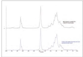
Figure 4. Unknown plasticizer spectrum vs. reference spectrum.
