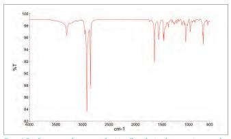
$\textit{Figure 8}. \ Baseline \ corrected \ spectrum \ of \ o-ring \ collected \ using \ the \ germanium \ crystal.$
