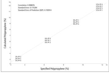
Figure 2. Calibration Model for PP
