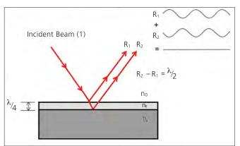
Figure 1. For an air  $(n_0)$  / film  $(n_t)$  interface, illustrated is the 180° phase shift between the two reflected beams  $(R_1, R_2)$ , resulting in destructive interference of the reflected beams.
