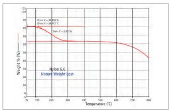
Figure 2. TGA results water wright loss for nylon 6,6.
