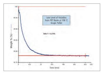
Figure 7. Low level emission of volatiles from single PET chip under gentle isothermal conditions at  $130\,^{\circ}$ C.
