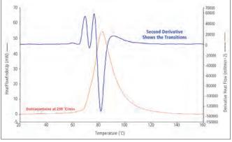
Figure 8. Heat flow of Dotriacontane, scanned with 250 °C/min.
