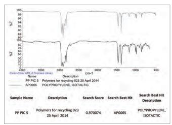
Figure 3. Search result identifying the sample as Polypropylene.
