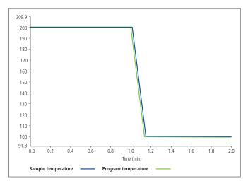
Figure 3. Sample temperature curve from DSC 8500 showing controlled cooling at 750  $^{\circ}\mathrm{C/min}.$
