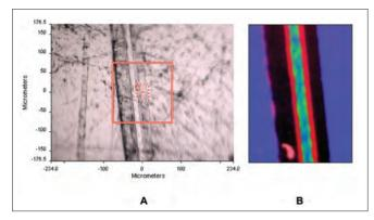
Figure 3. Visible and IR-reconstructed images from embedded laminate.
