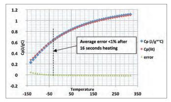
Figure 4. Specific heat capacity of sapphire using the 400  $^{\circ}\mathrm{C/min}$  heat-cool method, showing Pyris data, literature data and error.
