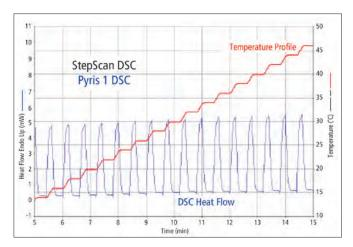
Figure 1. StepScan DSC approach using time-temperature profile.
