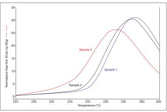
Figure 3B. The beta phase fusion effects of the systems 1, 2 and 3 (in 2005), i.e. heating rate 300  $^{\circ}$ C/min.
