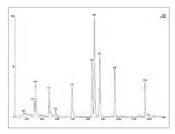
Figure 1. 50 ng injection of a reference standard for volatiles analysis by EN-71 with HS Trap.
