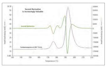
Figure 7. Carbamazepine heat flow and second derivative.
