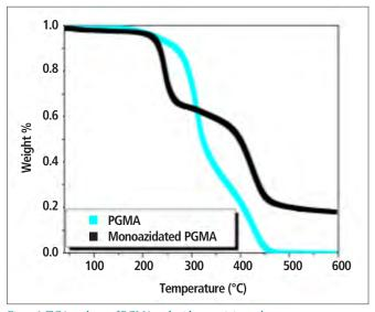
Figure 3. TGA analyses of PGMA and azide-containing polymers.
