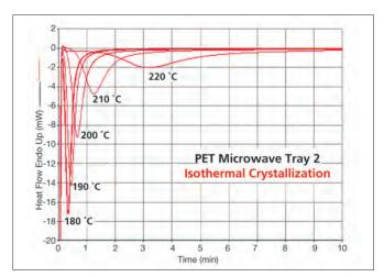
Figure 8. Isothermal crystallization results for PET Tray 2.
