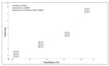
Figure 5. PE Calibration Plot of Peak Area vs Specified Concentration with Peak Area Ratio and Quadratic Regression Fit Type
