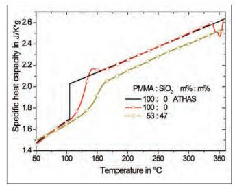
Figure 4. HyperDSC measurements at 400 K/min heating rate for pure PMMA and the nanocomposite filled with 47 m% spherical  $SiO_2$  nanoparticles. Sample mass 0.5 mg. The black lines represent reference data for PMMA from ATHAS<sup>4</sup>.
