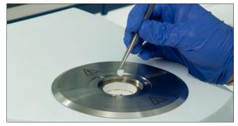
Figure 1. The TGA 4000 is a small rugged Thermogravimetric analyzer, available with and without auto-sampler, suitable for research grade work.
