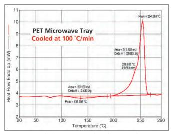
Figure 5. DSC results for PET tray resin after cooling at 100  $^{\circ}\text{C/min}.$
