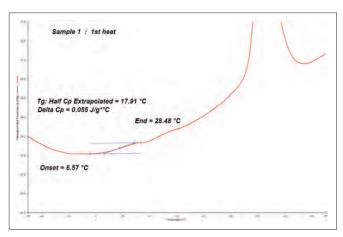
Figure 5. The DSC Tg value determination of sample 1 at 300 °C/min (in 2005).
