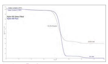
Figure 5. Detecting a filler in nylon
