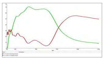
Figure 16. Transmission (green) and reflectance (red) spectra of thin film crystalline silicon deposited on a glass slide.
