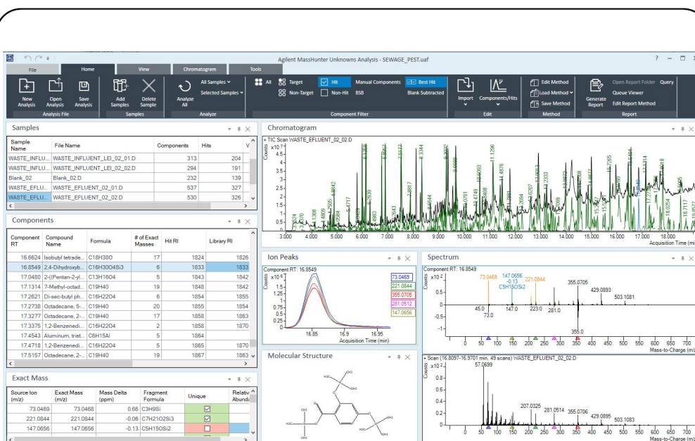
Figure 4. Unknowns Analysis B.10.00 and spectrum comparison with NIST17.
