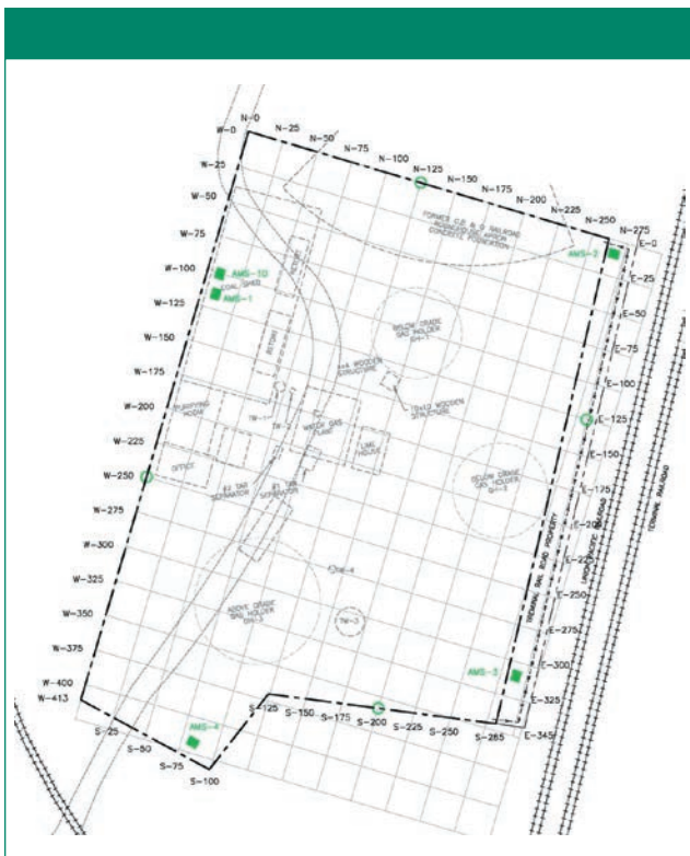
Figure 6: Layout of the MGP site. The sampling sites are shown in green
