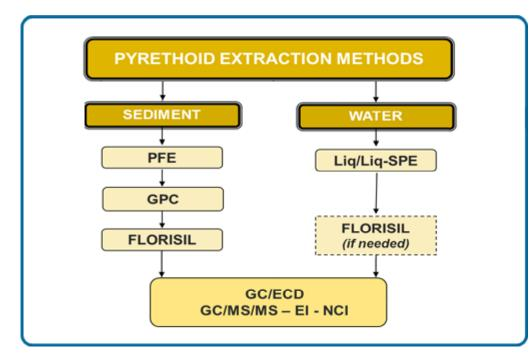
Figure 1: A flow diagram of the sample preparative procedure shows the differences between water and sediment. PFE is an abbreviation for Pressurized Fluid Extraction and GPC is an abbreviation for Gel Permeation Chromatography.
