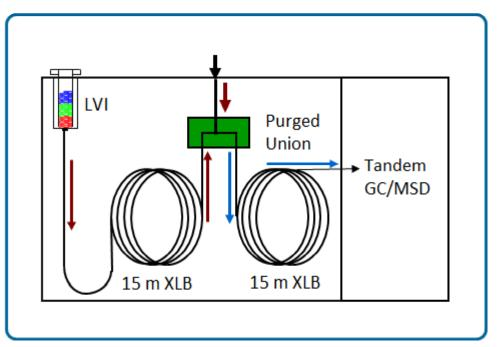
Figure 2: Tandem GC/MS system configuration with midcolumn back flushing.
