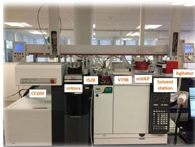
Figure 1: GERSTEL Dual Head MPS for fully automated derivatisation workflows for metabolomics applications
