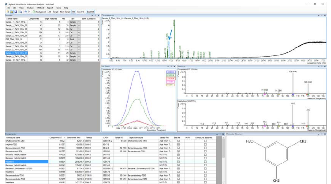
Figure 10: Using the Quantitative target list, Unknowns Analysis will first identify the target components then find and identify new components as Hits.
