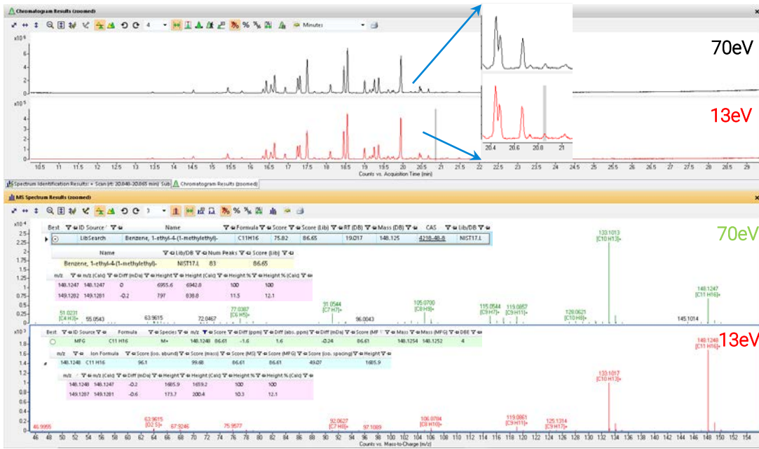
Figure 3: Comparing 70eV (above) and low eV (below) for a low level component with mass accuracy maintained.
