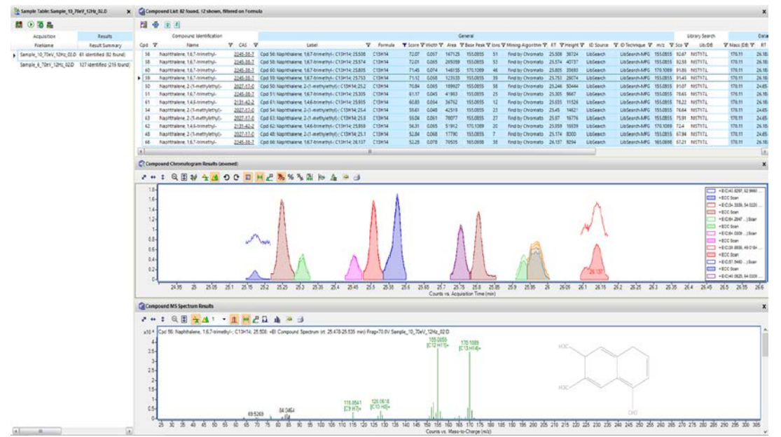
Figure 5: Molecular Feature Extraction and NIST17 library searches provided quick identification of C3-naphthalenes.
