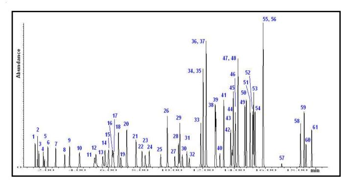
Figure 1. Volatiles at 20 PPB concentration purged from water.
