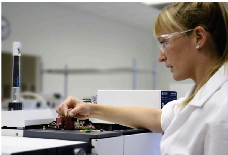
Figure 5 - The 5800 Sorbent Pen Desorption Unit (Entech Instruments) was installed on a 7890/5977A, allowing split or splitless desorption of the Sorbent Pens into the GCMS.
