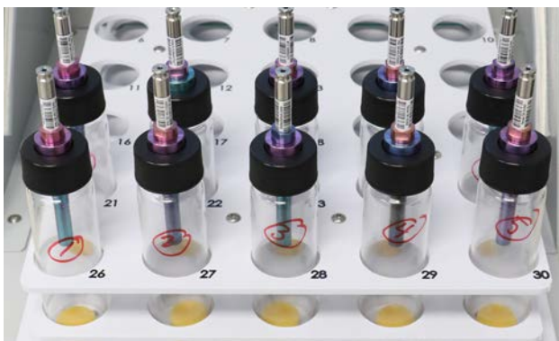
Figure 1 - The vacuum tight seal allows samples to remain under vacuum after a 30 second evacuation, allowing elevated rates of static diffusion to collect significantly more headspace compounds on the adsorbent than can be collected at atmospheric pressure. Sorbent Pens are all labeled with a barcode sticker. This allows the operator to simply scan each Sorbent Pen into the sequence table to record its identity and track each Sorbent Pen through its lifetime of hundreds to thousands of extractions and desorptions.
