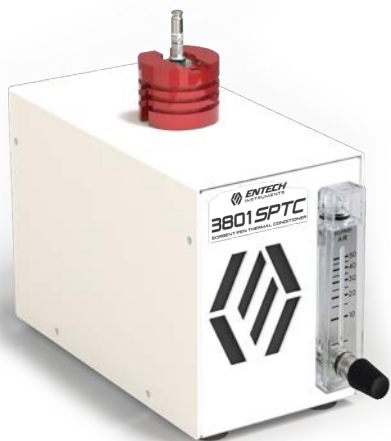
Figure 3 - To prepare new Sorbent Pens for extraction, the 3801 Sorbent Pen Thermal Conditioner (SPTC) is used to condition Sorbent Pens prior to use up to 300^\circ\text{C} depending on the sorbent type. During the analysis, the Sorbent Pens are both desorbed to the GCMS and thoroughly baked out, eliminating the need for additional thermal conditioning before reuse. However, if a Sorbent Pen was not isolated after extraction or if it contained unusually high concentrations of extracted compounds not completely removed during the previous analysis, the 3801 SPTC can be used for a quick cleanup of the Pen.
