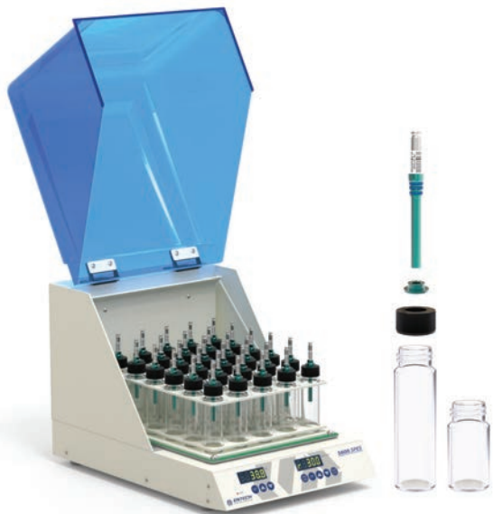
Figure 4 - Sample vials and agitator used to perform VASE. The 5600 Sorbent Pen Extraction System (SPES) provides a convenient way to perform vial extractions using 30-position trays, allowing for significant sample throughput. The sample to be extracted is loaded into the vial, the Sorbent Pen is inserted, a vacuum is created through the MicroQT seal at the top of the Pen, and the sample is loaded onto the tray. The extraction time, temperature, and RPM can be programmed on the 5600 SPES and the vacuum extraction process begins. The Sorbent Pen Extraction System agitates the samples at 30-300 RPM to speed up transfer of volatiles to the headspace, while heating the sample from ambient +4°C to 70°C. Extractions can be completed in 1–48 hours depending on the application. Extraction times for this study were 2-15 hours.
