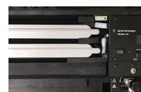
**Rechargeable batteries** provide up to 8 hours of operation. It is possible to switch to an external power supply when available.
