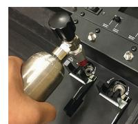
A supply of operational gases with up to two **refillable gas canisters**, user configurable as dual carrier gas or double volume. The use of quick connectors enables one-click exchange.
