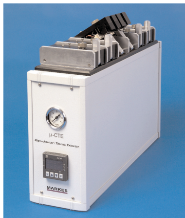
Figure 4: Markes Micro-Chamber/Thermal Extractor ( \mu -CTE) for simultaneous sampling/purging of 6 material samples - in this case, sand
