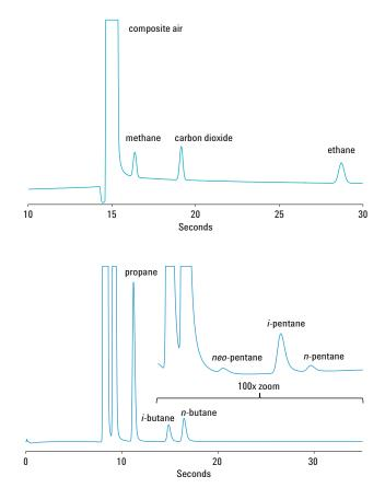
Figure 2. Fast and simultaneous analysis of well gases on two independently controlled column channels.
