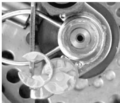
Figure 4. Residues from standard septa inside injection port.
