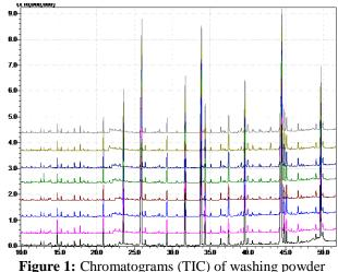
figure 1: Chromatograms (TIC) of washing powder for the determination of the repeatability.
