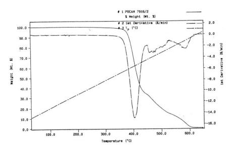
Fig. 1. TGA-plot of the polymer blend.
