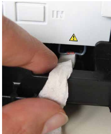
Fig. 13: Drying the leak sensor
