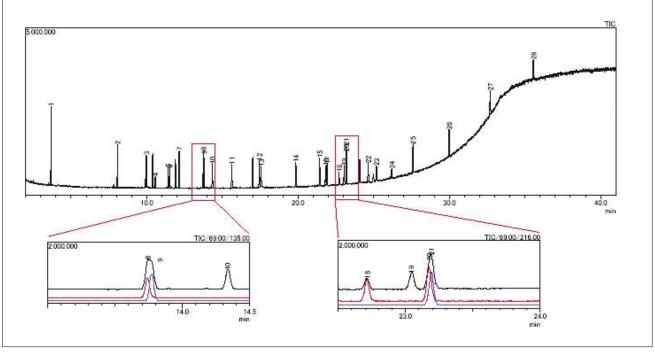
Fig.1 TIC of SCAN Mode (10ppm sample)
