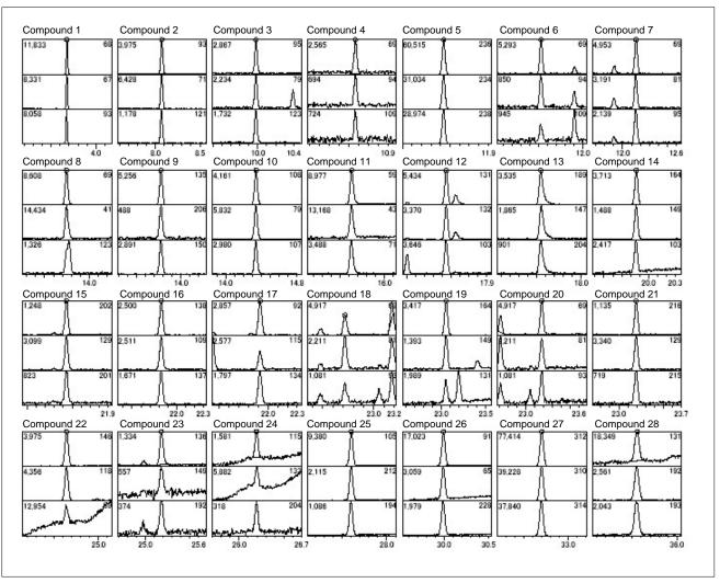
Fig.2 Mass Chromatograms of SIM Mode (0.5ppm samples)
