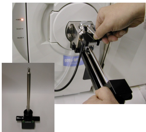
Fig. 1: Direct Sample Introduction Probe (Bottom Left) and Insertion of the Probe into the MS Unit
