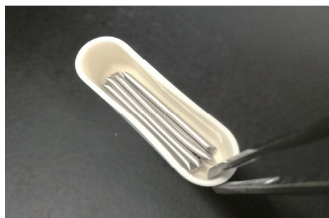
Fig. 3 Stainless Steel Pipes in the Sample Boat
