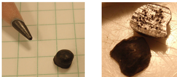
Fig. 1 (Left) Approx. 5-mm Diameter Plastic Pellet (Right) Cross Section
