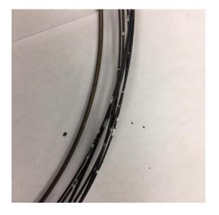
Column continuously exposed to temperatures above its temperature limit
