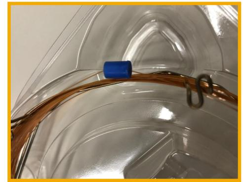
Column plug holds column ends together and protects against contamination. To put the column in storage, use this plug again or a piece of septa over the ends of the column.
