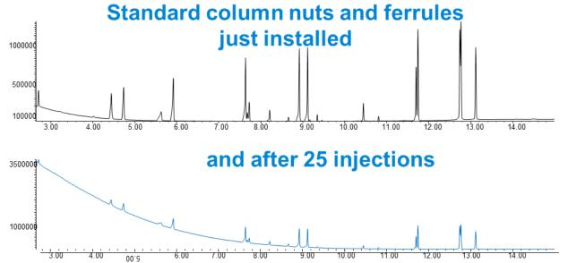
Frequent retightening of the fitting is needed to maintain a leak-free seal, as well as system performance and productivity.
