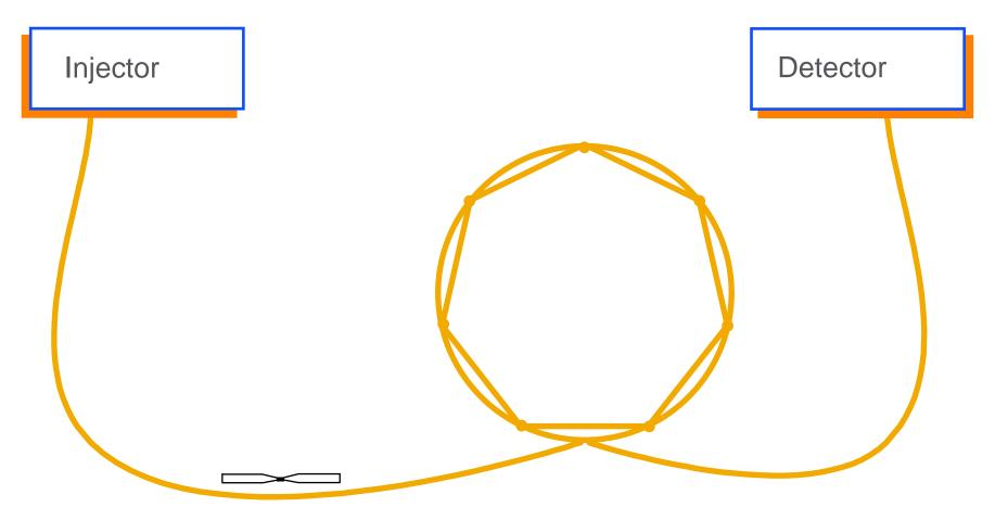
The guard column is 3–5 m of deactivated fused silica tubing with the same diameter as the analytical column. It is connected with a zero dead volume union.
