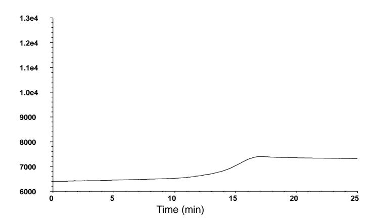
Temperature program the column without an injection\*
