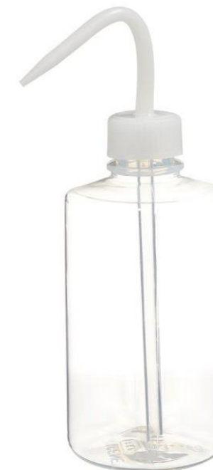
Teflon wash bottle, best for ppt level preparations
