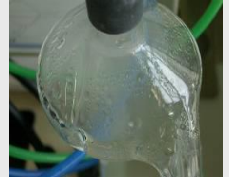
Dirty spray chamber
