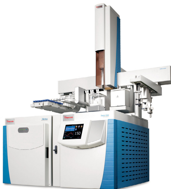
Figure 1. TSQ Duo GC-MS/MS system with Thermo Scientific ™ TriPlus RSH ™ Autosampler.
