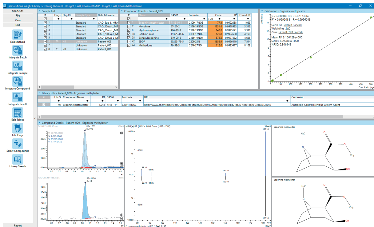
Figure 4. Using LabSolutions Insight software to review data acquired with unknown patient samples, both MRM triggered product ion spectrum and MRM Spectrum mode deliver the same quantitative data quality compared to a validated conventional 2-3 MRM method.
