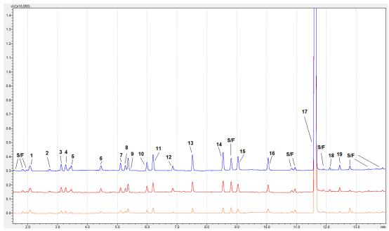
Figure 1: Comparison of the FID Chromatograms of the 1 L Mixed Standard diluted in 1000 mL (Bottom), 500 mL (Middle) and 250 mL (Top) of Internal Standard. The numbers correspond to the compounds in Table 4. The S/F indicates that this peak was part of the system/film background.
