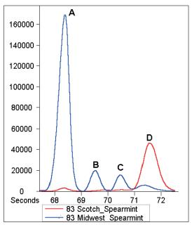
Figure 2. Extracted Ion Profile Chromatogram Overlay of m/z 83 in Scotch and Midwest Spearmint Oils.
