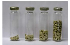
Figure 1 – Comparison of 1 g, 2g, 4g, and 8g of a HT Polymer Sample in 22 mL High Temperature Headspace Vials
